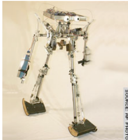
The walking robot Cornell moves like a human, falling and catching itself as it moves forward.
